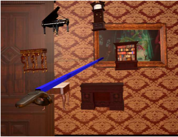
Figure 1: The user receives a video feed of the real environment from the front camera of the HTC VIVE. That enables the user to choose which physical objects to substitute for inclusion in the Virtual Environment.
